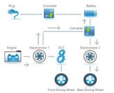
4WD: When more power is needed, the gas engine and the electric motor (M2) power the vehicle together. If the accumulated power is much enough, the gas engine will also drive electric motor (M1) to charge the battery pack. As speed increases, the gasoline engine can take over seamlessly with support from the 6-speed DCT; when braking, the gas engine automatically shuts down and the electric motor (M2) takes over.
